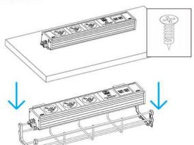
2. Fixate using one Philips screw M3x18 on each side
